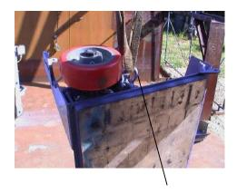
Pick up the magnet/ drive assembly with a fork lift, strap and shackle. Locate the shackle around the threaded rod, as shown, so the unit will hang in a vertical and balanced position.
