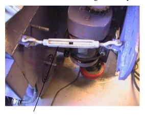
Swing the magnet assembly around and attach the turnbuckle as shown.
