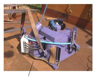
Using a fork lift, strap and shackles, lower the machine on its back side as shown.
