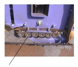
Remove the magnet mount by loosening the lock down bolts.
