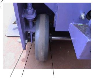
With the unit still lifted slightly off the floor, remove the (3) split collars that hold the front tires in place. Remove the axle and tires.
