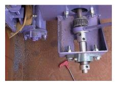
Slide the control cage arm off of the cog hub by loosening the retaining collar and rocking the arm back and forth until it comes off.
