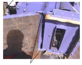
Remove the two  $\frac{1}{2}$ " bolts at the hinge pivot Points and remove the magnet assembly.
