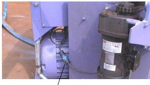
Swing the magnet around and disconnect the magnet drive power cord.
