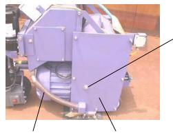
If the cover plate doesn't remove easily, remove the ½" nut which holds the side liner in place. Then remove The cover plate and pry the Liner out of the cabinet opening.
