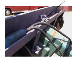
Make sure that the cord grip loops are secured to the hoist frame so the cables cannot be pulled loose at the motors.
