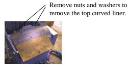
To remove the liners at least 3 wheel blades must be removed to allow clearance to get the liners out. Remove the back wall liner first by removing the nut and washer on the front of the blast cabinet. Then remove the top curved liner by removing the two nuts and washers on top of the blast cabinet. When replacing the liners make sure they are seated properly and are tightly secured.
