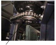
Torque Tamer Assembly-Pt#110 Includes sprocket & Spacer
