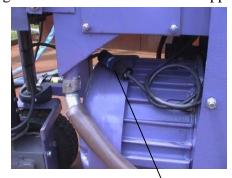
Plug in the rear tire drive. Make sure that the white coded plug is attached to the white coded receipt.
