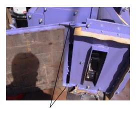
Place the magnet pivot eye mounts on top Of the wall blast plate mounts and attach with (2) ½" bolts and lock nuts.
