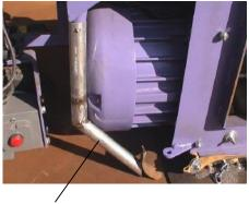
Remove the reclaim drain/ dribble valve
