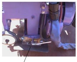
Lift the machine a few inches of the floor, with a fork lift, strap and shackles- see lifting points page . Remove the seal assembly by removing the nut and chain attachments on both sides of the machine.
