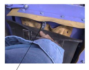
Attach the seal by sliding the chain onto the mounting stud and securing with the lock nut. Follow the same procedure to secure the bottom.
