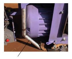
Attach the reclaim drain/ dribble valve
