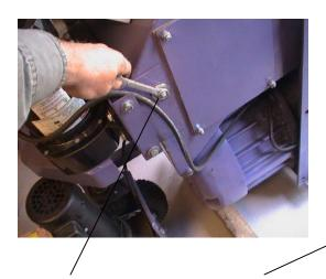
Loosen the nut holding the side bracket And remove the steering assembly.
