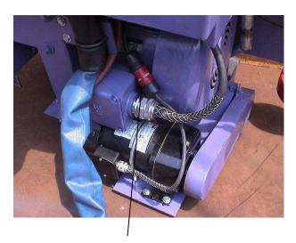
Plug in the screw drive motor. Make sure the Red coded plug is connected to the red coded Receptacle.
