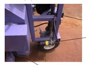
Place a 4x4 under the blast motor and lower the unit back down on the floor.
