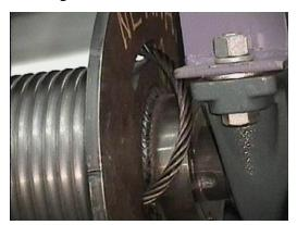
Pull the cable through the drum and out the Hole in the opposite side. Then clamp the Cable in the welded saddle as shown.
