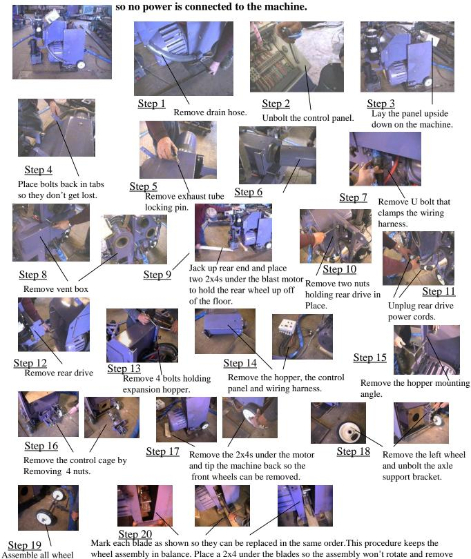
Mark each blade as shown so they can be replaced in the same order. This procedure keeps the wheel assembly in balance. Place a 2x4 under the blades so the assembly won't rotate and remove all 8 blades. Use a breaker bar and 3/4" socket to loosen both bolts first, then use a ratchet to remove the bolts. Both bolts must be loosened first so you don't strip threads while removing the bolts.
