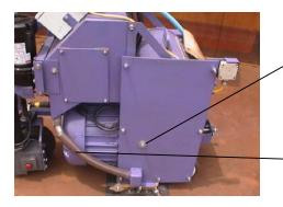
Set the side cover plate in place over the liner stud. Install The ½" lock nut and washers on the liner stud and the (7) ½" bolts and lock nuts around the cover.. Tighten all bolts securely.
