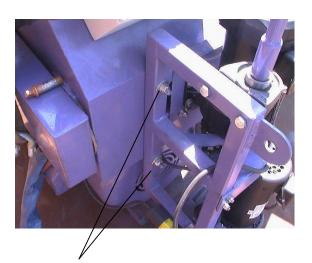
Place the steering assembly on the two studs located on the reclaim hopper. Install washers and lock nuts and tighten.
