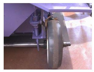
Lift the unit back vertical. Holding the unit slightly off the floor, slide the axle and right tire assembly through the adjustable support.
