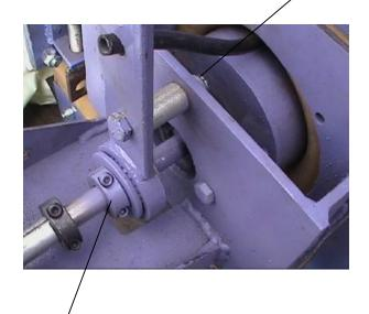
Loosen the collar and slide the collar and washer back away from the adjustment locking arm.
