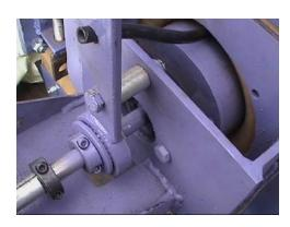
After making the changes slide the locking arm back in place and and Install the locking bolt, collar and washer.
