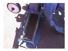
Slide the seal assembly under the blast cabinet opening.
