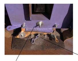
Make sure that the lower liner is in place and bolted securely.
