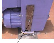
Set the side liner in place as shown.flush with the cabinet wall. Use tape to hold the top if required.
