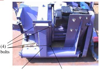
Remove the (4) ½" bolts holding the lower reclaim assembly in place. Remove the lower reclaim assembly.
