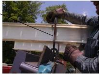
Make sure that the hoist support brackets are mounted as close to the front tires and vertical support beams as possible. Additional holes are provided in case the hoist has to be moved out further from the tank wall so the cables can clear vents are other obstructions. When the hoist is moved out, addition counter weights will have to be added to the back end of the fixture. Bolt the brackets down to the beam with (4) 5/8" grade 5 bolts.
