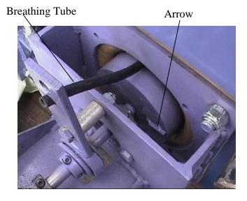
Rotate the control cage clockwise until the arrow on the end of the control cage is at 3:00 to 5:00. Be sure to reinstall the breathing tube.
