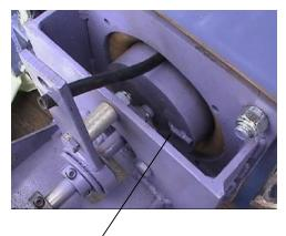
Rotate the arrow on the control cage to 3:00 (as shown) for vertical cleaning.
