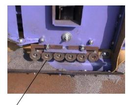
Slide the magnet mount in place as shown. Secure with lock down bolts.
