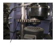
Steering Shaft Assembly-Pt#107 Includes-Sprocket,lower Bearing & gearbox mount
