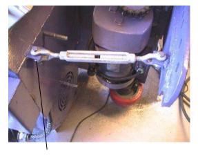
Remove the turnbuckle bolt from the reclaim hopper.
