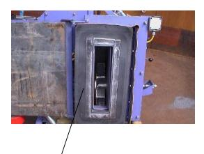
Place the seal on the wall blast plate as shown.
