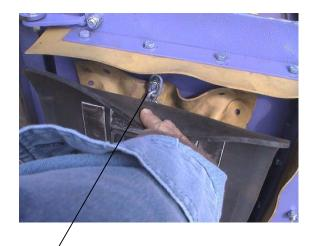
Remove the lock nut holding the seal Chain support from both the top and Bottom of the seal assembly.
