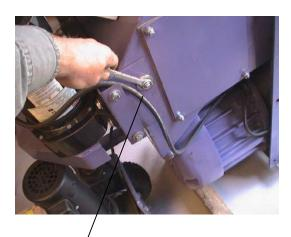
Tighten the lock nut on the side support plate.
