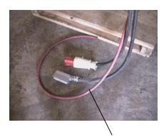
An air hose is included in the machine wiring harness to provide air power for options we will offer in the future. The air disconnect on the dust collector is not used now, but will be used to connect the air line in the future.
