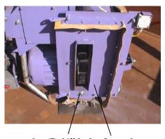
Remove the (7) ½" bolts from the wall blast plate and the nut and washer holding the bottom liner in place.
