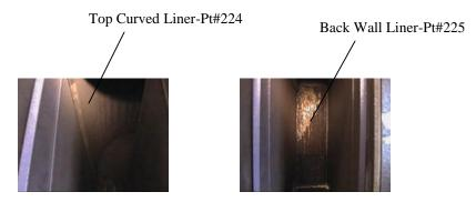
There are two liners in the machine that are used in the machine for both horizontal and vertical operation- the Top curved liner and the back wall liner. Inspect these liners for wear at 50 hour intervals. If wear is found, remove the liners and fill the wear area with hard face weld. If the wear is too great, replace the liner.
