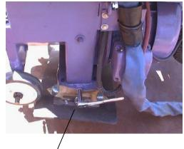
Attach the seal assembly. Slide the attachment chain over the stud and secure with a lock nut. Then secure the attachment chain on the other side of the machine.
