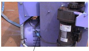
Connect the magnet drive power cord. Make sure the blue coded plug is matched with the blue coded receptacle.
