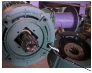
5. Slip the brake assembly off of the motor shaft being careful not to pull on the brake electrical wires. Use bailing wire to support the brake so no stress will be put on the wires while you clean the brake.
