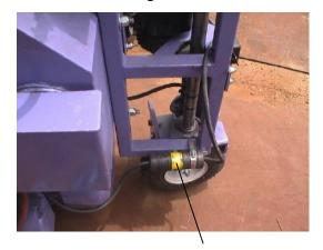
Plug in the steering motor power cord.
