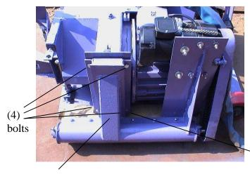
Slide the lower reclaim assembly in place over the blast cabinet opening as shown. Attach with the  $(4) \frac{1}{2}$ " bolts and lock nuts.
