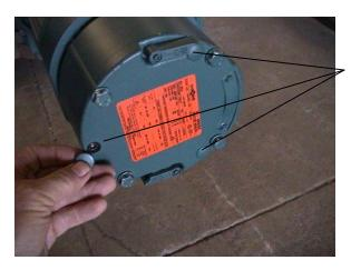
Remove the three plugs on the end of the brake. Tighten each of the three Allen head bolt ¼ turn and try the hoist again. Continue this procedure until the brake works properly.
