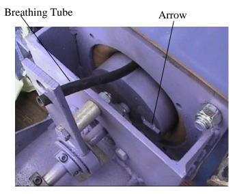
Rotate the control cage counter clockwise until the arrow on the end of the control cage is at 10:00 (3:00 is shown in photo). Be sure to reinstall the breathing tube.
