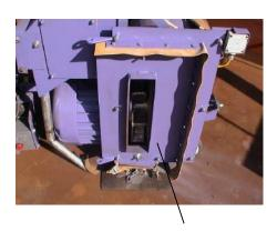
Bolt on the wall blast plate using the (7)  $\frac{1}{2}$ " bolts from the side cover plate.
