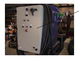
Main Control Panel is located on the dust collector. It controls all machine functions.
